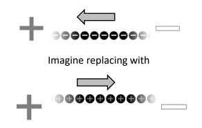
Replacing real negative electrons with imaginary positive charges flowing in the other direction to make conventional current
