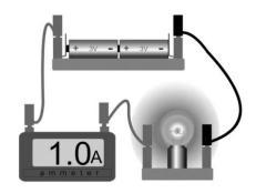
Connecting an ammeter so all the current flowing through the bulb has to flow through the ammeter, too
